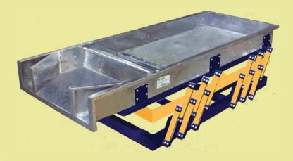
SHIFTEA - Green Leaf Shifter is a well proven machine for shifting the Kutcha leaf. It serves as a feeder for Rotorvane and CTC machines. The machine is fitted with a stainless steel perforated tray. Leaf fed onto the tray moves in a series of hops thereby shifting, cooling & breaking the lumps' in leaf and also separates any foreign matter and dust from Tea leaf. The machine is noiseless and vibration free.
